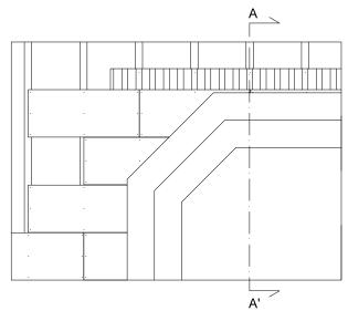
Xlam wall structure made of solid wood panels with crossed layers, composed by several layers of lamellas (or boards), overlapped and glued one on the other so that the grain of each single layer is rotated in the plane by 90 ° with respect to the adjacent layers.
